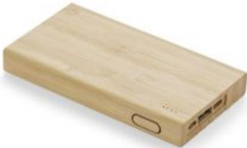
SILVA is an environmentally friendly power bank with a capacity of 8000 mAh. It was closed in a housing made of 100% bamboo. Standard micro USB charging cable included. The product complies with all the relevant European Union directives, has the CE mark and 1 year warranty. Technical data: input (micro USB and USB type C) 5V / 2A, output USB 5V / 2A, ion-polymer battery.
