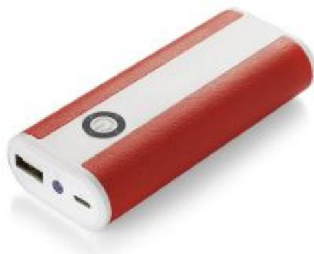
REMOTE is a power bank with capacity of 5200 mAh. Gadget's sides are covered with eco leather. Power bank have build-in micro USB cable, flashlight with two modes (continuous and flashing) and 4 leds showing the battery power level. Input 5 V / 1 A, output 5 V / 1 A (integrated cable) and 2.1 A (USB port). Micro USB cable attached.
